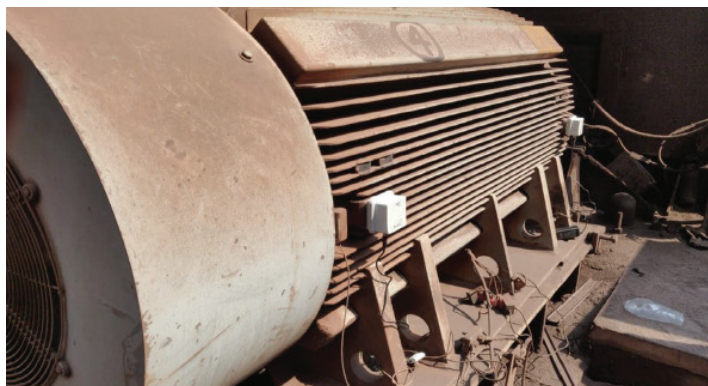
Sensors installed on Drive and Non-Drive End of a Motor
