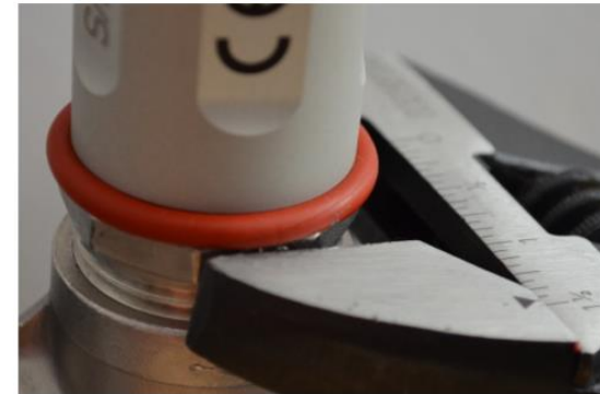
Figure 3-4 Correct tightening of the device
