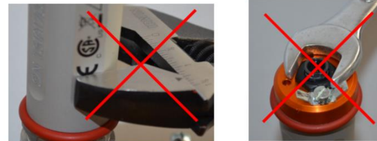
Figure 3-5 Incorrect tightening of the device
