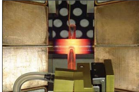
Thermal Cycles and Heat Treatments: Many different grips are available to support uniform temperature zones and a variety of specimen configurations. Other grips can be used to provide thermal gradients in the specimen for weld HAZ and process simulation.
