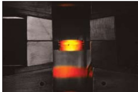
Melting and Solidification: Melting and controlled solidification can be performed in-situ. Thermal and mechanical testing of the as-cast structure can then be performed to identify cast structure properties and ductility dip regions.
