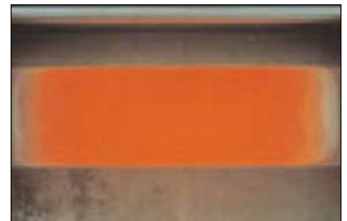
Strip Annealing Process Simulation: Both batch and continuous annealing processes can be simulated using a strip annealing jaw system.
